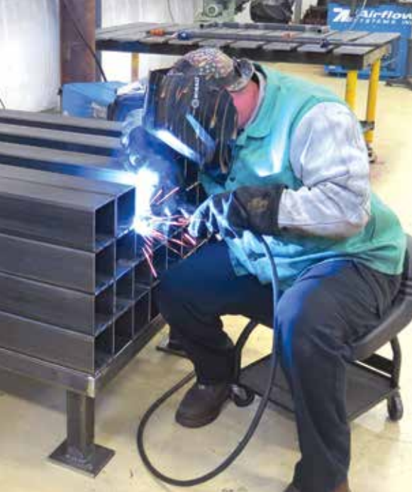
A Daman Continuous Improvement team member welds tubes for Cell C.
