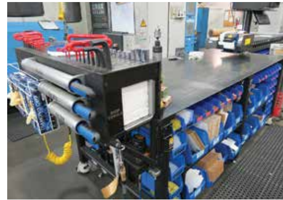
This workbench was customized by the Continuous Improvement department to reduce clutter and organize tools in order to streamline productivity.
